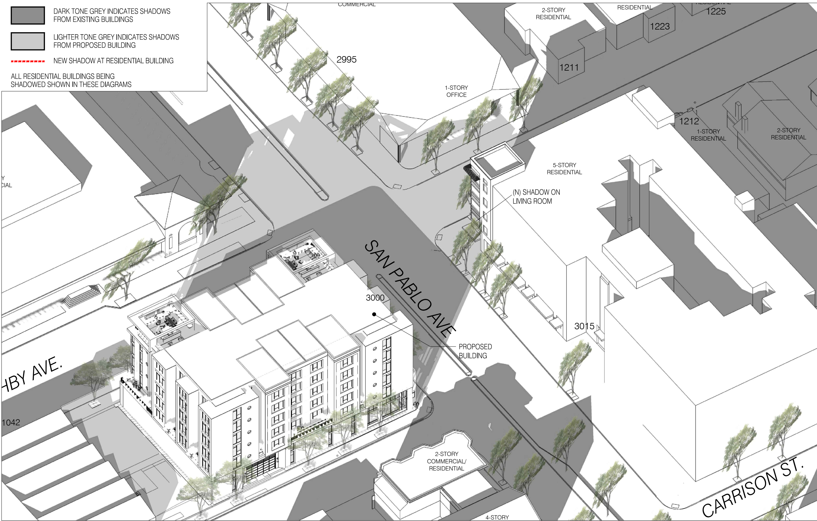
4 SHADOW STUDY AXONOMETRIC - DEC 21: 2-HRS BEFORE SUNSET NTS
